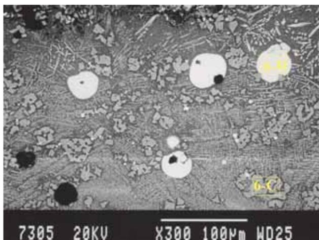
Figure 17 SEM image of the matrix of slag No. 6.
