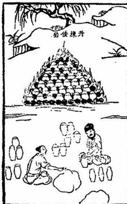
**Figure 1** Drawing of the zinc-smelting process recorded in *Tian Gong Kai Wu*.
