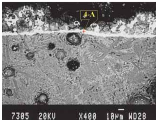
**Figure 14** SEM image of the matrix of slag No. 4, high zinc content at position 4A.
