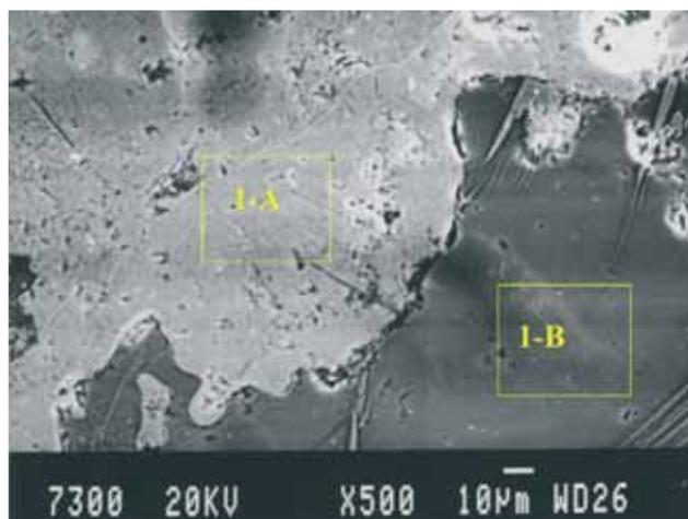
**Figure 11** SEM image of polished section of slag No. 1 adhered to retort wall, high zinc content in white area 1A (see Table 1 for analyses).
