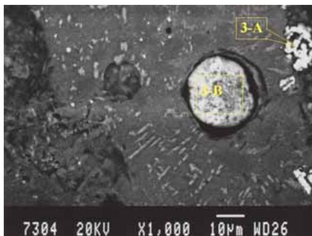
**Figure 13** SEM image of slag No. 3 adhered to retort wall with zinc-rich area 3B.
