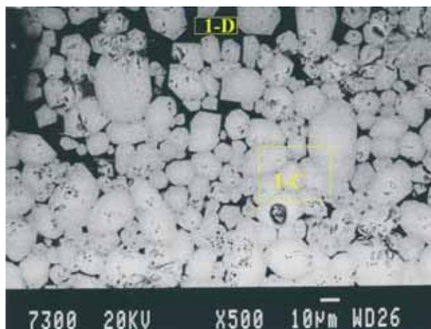
**Figure 12** SEM image of slag No. 2 adhered to retort wall, high zinc content in white area 1C.
