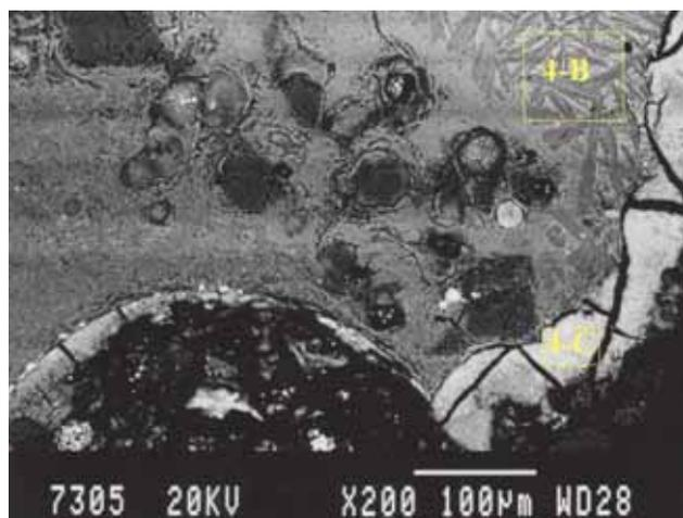
**Figure 15** SEM image of the matrix of slag No. 4 with high zinc content at 4C.
