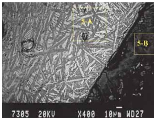
**Figure 16** SEM image of the matrix of slag No. 5.
