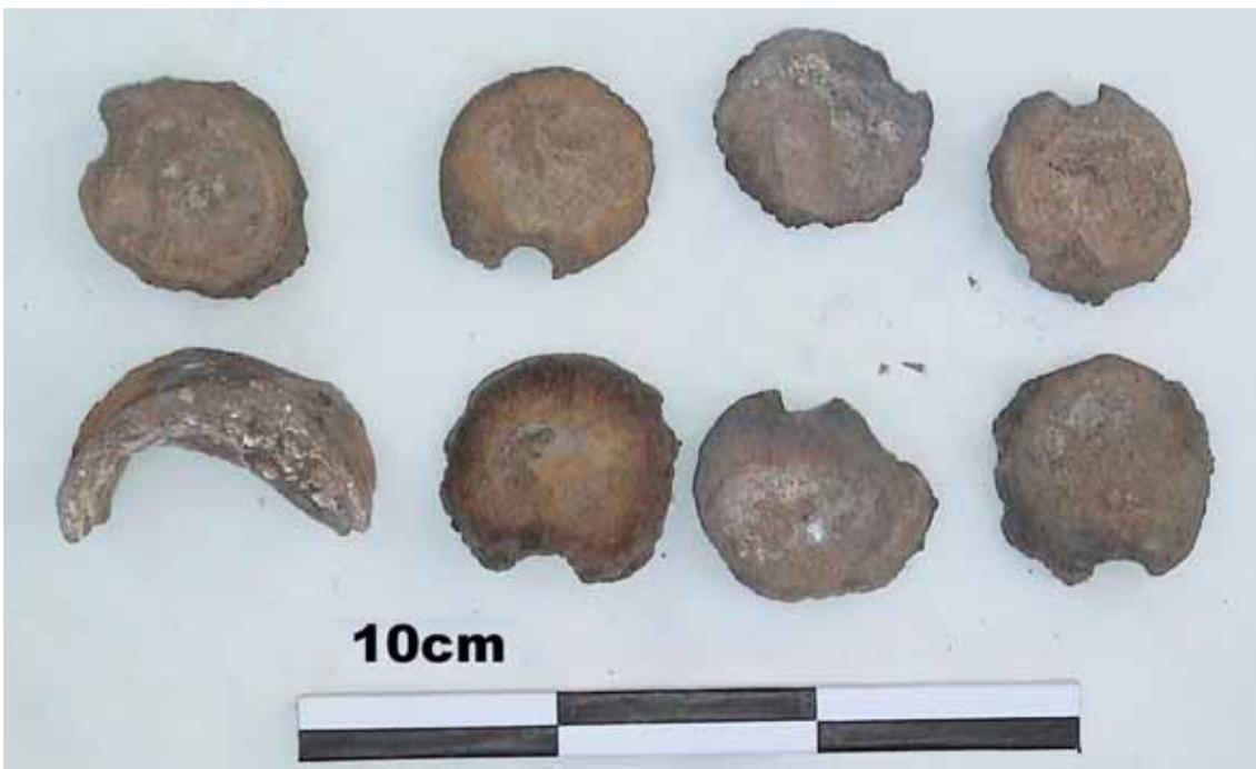
Figure 7 The pockets for collecting the zinc at the top of the retorts.
