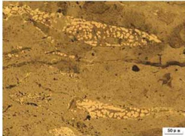
Figure 4: The microstructure of a bloomery iron object excavated from the Ili Valley, Xinjiang
