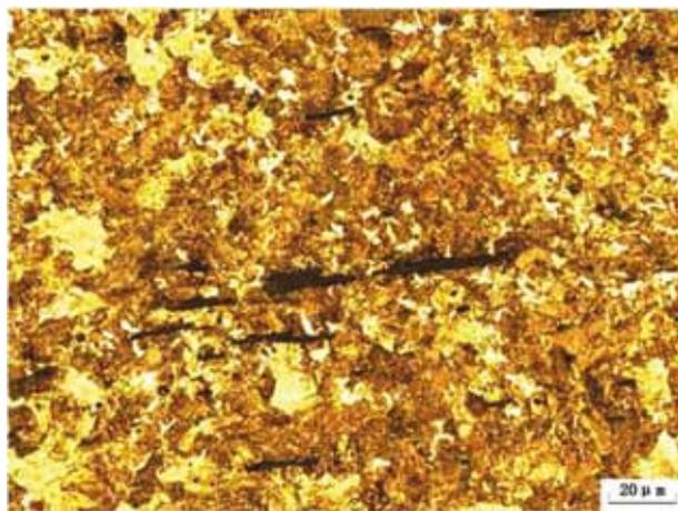
Figure 12: The microstructure of a puddling steel sword excavated from Suizhou, Hubei province.
