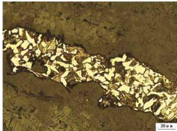
Figure 5: The microstructure of a carburised steel object excavated from the Ili Valley, Xinjiang.
