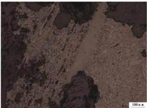
Figure 7: The microstructure of the iron bar excavated from tomb M444 at the Mogou site, Lintan county, Gansu province.
