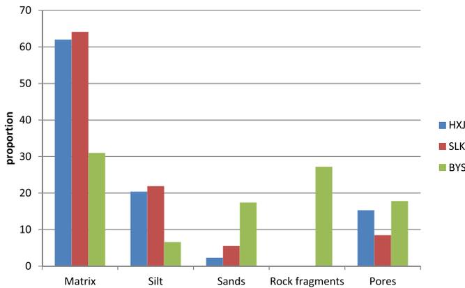
**Fig. 10.** Comparison of petrographic microstructures from HXJ, SLK materials and BYS linings.
