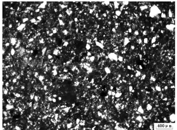
Fig. 7. SLKH100, 25X, XPL, furnace wall, clay bricks, clay matrix is nearly 70% with silt balance.
