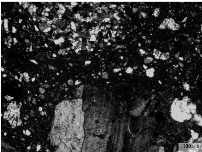
**Fig. 8.** BY511Y3:9, 10X, XPL, furnace lining, with very small proportion of clay matrix, indicating the addition of sand, and showing gravel sized rock fragments.
