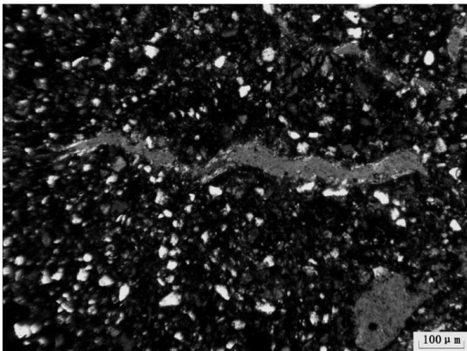
Fig. 6. HXJFM5, 10X, XPL, furnace wall, rammed clay, clay matrix is nearly 70% with silt balance, a pore in a long-formed shape.
