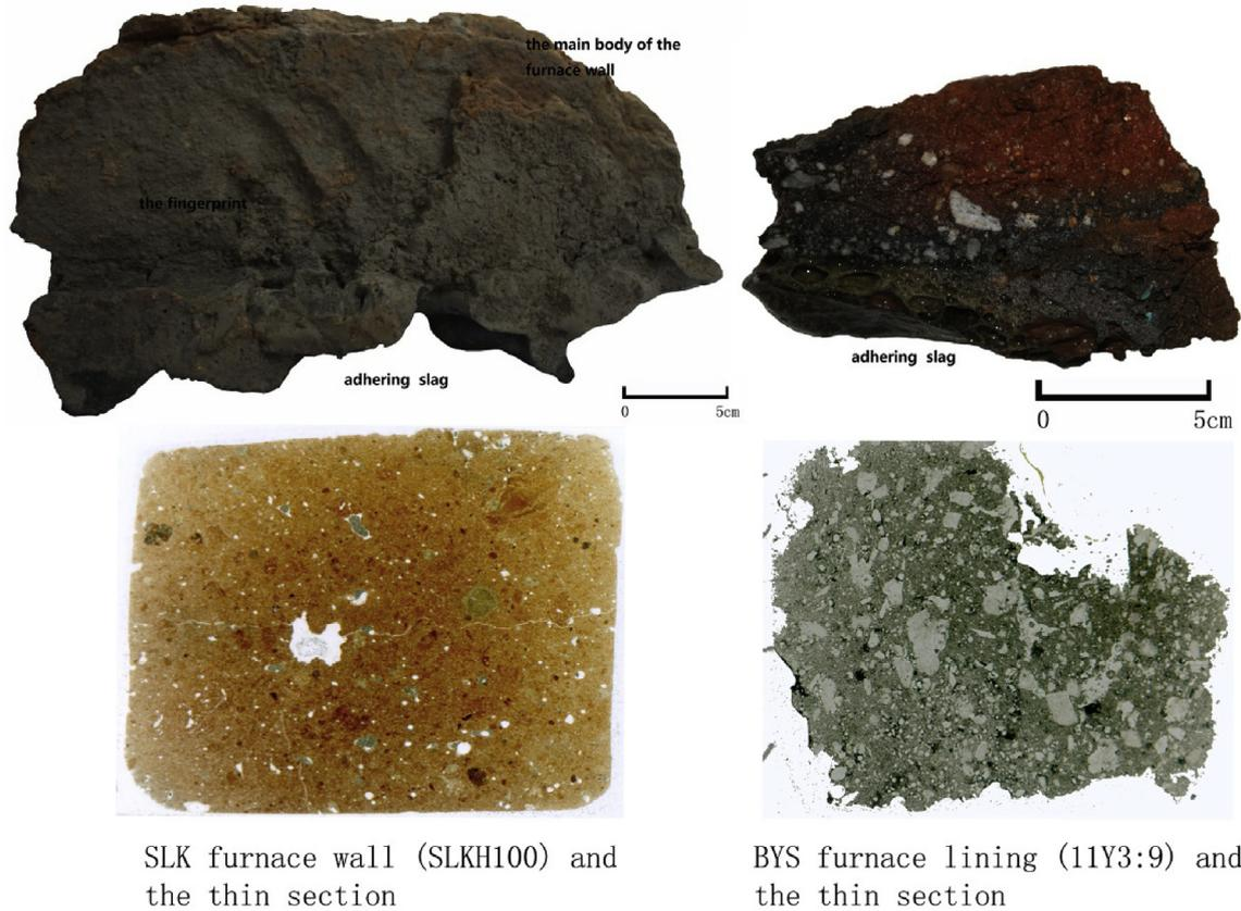
Fig. 5. Furnace materials from the SLK site (left) and the BYS site, showing different macrostructures representative of their respective furnace material.
