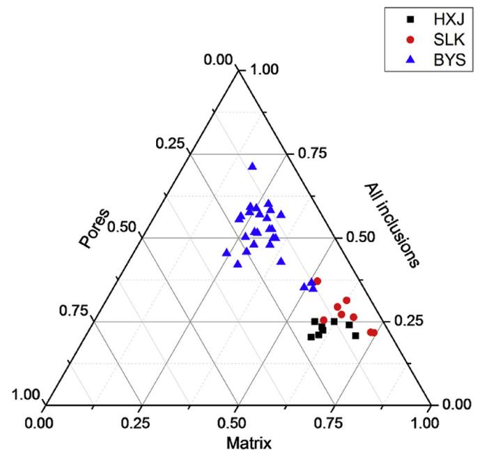
**Fig. 9.** Ternary diagram showing point counting results of HXJ, SLK walls and BY5 linings.
