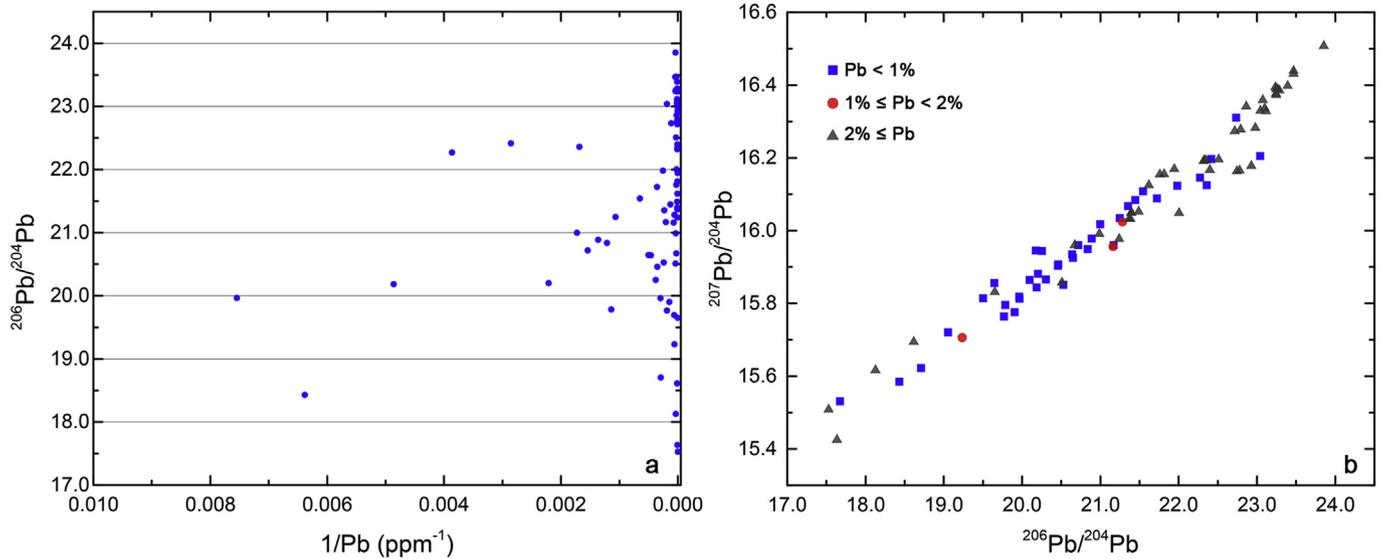
Fig. 3. (a) A plot of Hanzhong bronzes data, showing 1/Pb against lead isotope ratio <sup>206</sup>Pb/<sup>204</sup>Pb. (b) A <sup>207</sup>Pb/<sup>204</sup>Pb versus <sup>206</sup>Pb/<sup>204</sup>Pb diagram for Hanzhong bronzes showing the distribution of lead isotope ratios of artefacts with different lead contents.
